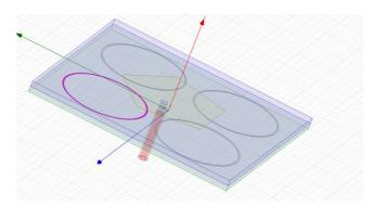
Fig 3. EBG unit cell for 5.8 GHz.
